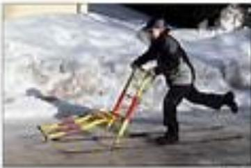
Have you heard about the kick sled? – a wonderful invention from Finland that has been around for over eighty years. These sleds can be used on hard surfaces, packed snow and ice. One foot stays on the ski and the other foot kicks to push off and send the sled sliding forward. In Scandinavia and Finland they are used as a form of transportation and in more remote areas, to buy groceries. There's a seat on the front.
